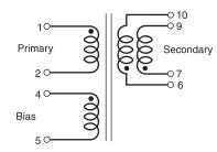
Secondary windings to be connected in parallel on PC board
